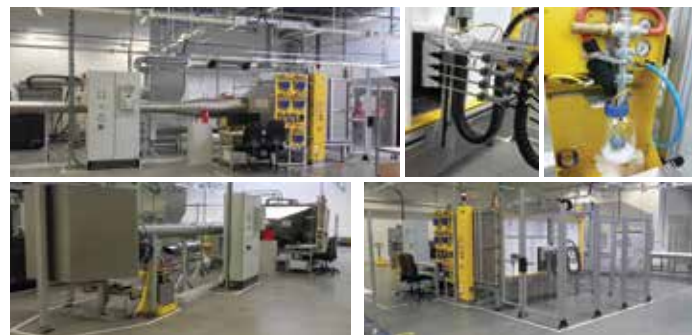
Typical HEPA/ULPA Auto-Scan Equipment
