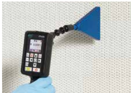
ATI's iProbe, Paired with a Photometer, Scans HEPA Filters to Detect Leaks
